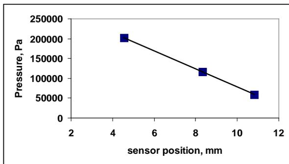
Data was obtained for Newtonian Glycerol at 1,220 s<sup>-1</sup> using a type C Sensor Chip. (1) Reference: K. Walters, Rheometry, Chapman and Hall, London, 1975.
